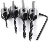
Unlike ceramic tiles that are only glued to the wall, the continuous flow seamless installation requires a combination of glue and countersunk screws. The tiles cannot be installed solely with glue. Using a countersink drill bit drill four holes near the four corners in the flattest areas of the 3D surface.
